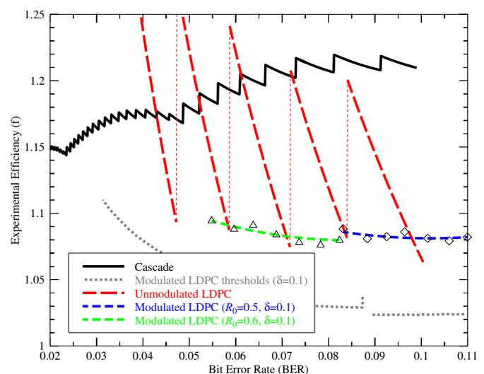
Fig. 1: Experimental efficiency for *Cascade*, and LDPC codes.
