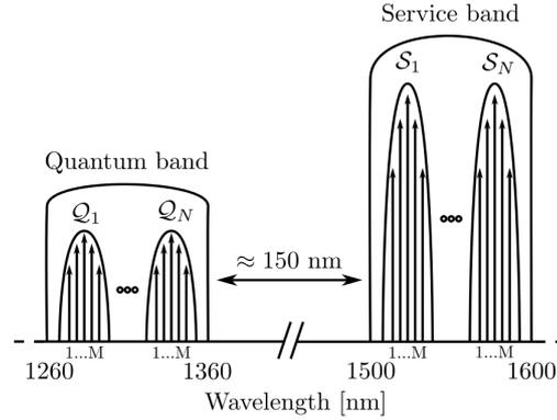
use of not only one channel per port, but also its periodic “harmonics”. Therefore, we slice the quantum and service bands in subbands that match the periods of the AWG, such that each QKD pair can use such periodically matching channels from both bands to communicate. The scheme is easily implemented using standard commercial components. A test bed network of three access networks and a span of 16 km has been deployed in order to test this scheme.
